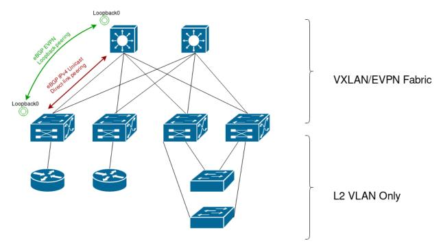
The top layer consists of the core (or spine) switches, each of the core switches will connect to all of the distribution switches forming a full mesh between core and distribution. Core switches does not have any other connections, no connections between two core switches and no external connections.
